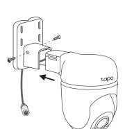
The camera is **not waterproof** when set on a table or shelf. Mount the camera via Option 1~3 when installing outdoors.
